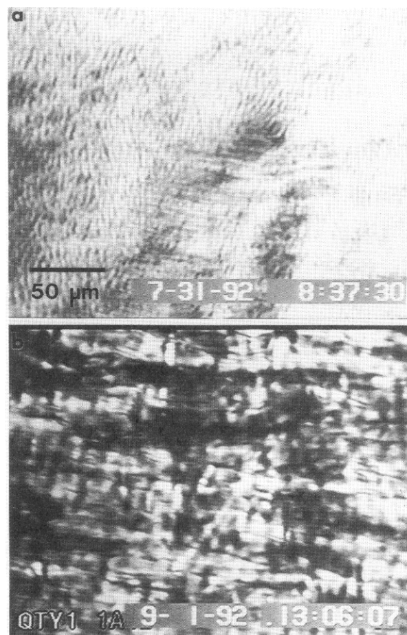
Figure 7. Polarized optical micrographs showing the evolution of texture while holding the specimen temperature at 80 °C. (a) The quenched-in fine-scale banded texture immediately after applied shear. (b) The coarsened texture after 1 month at 80 °C.
